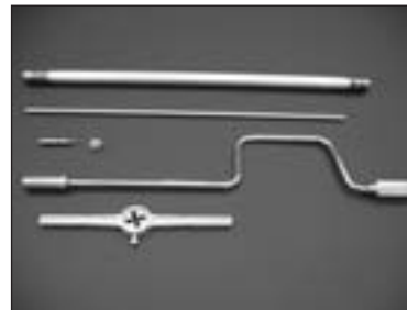
D-2 installation socket, D-2 hex nut alignment tool, speed wrench, die and diestock
